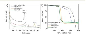
Fig. 1 (a) XRD patterns ( $CuK\alpha$ ) of the three composite materials Rh(nP)/nC (blue trace), PtRh(nP)/nC (orange trace), and Pt(nP)/nC (green trace) in comparison to the carbon starting material (nC, black trace). (b) Thermogravimetric analysis (TGA) of the three composite materials and the starting carbon material between 50–800 °C under synthetic air (80%  $N_2$ , 20%  $O_2$ ) with a heating ramp of 10 °C min<sup>-1</sup>.
