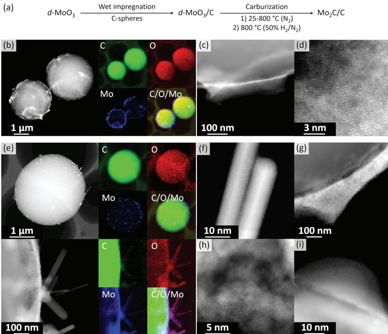
**Fig. 1** (a) Synthesis of  $\beta\text{-Mo}_2\text{C/C}$  from delaminated  $\text{MoO}_3$  films; (b) HAADF-STEM images and EDX maps of  $d\text{-MoO}_3/\text{C}$ ; (c) and (d) HR-STEM images of  $d\text{-MoO}_3/\text{C}$ ; (e) HAADF-STEM images and EDX maps of  $\beta\text{-Mo}_2\text{C/C}$ ; and (f)–(i) HR-STEM images of different morphologies decorating the surface of carbon spheres in  $\beta\text{-Mo}_2\text{C/C}$ .
