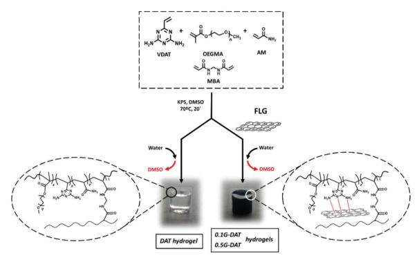
Fig. 1 Synthesis of DAT and G-DAT hydrogels.
