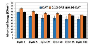
Fig. 7 100 cycle fatigue test for (G)-DAT hydrogels.
