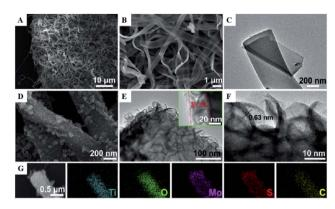
Fig. 11 (A) Low, (B) high-resolution FESEM, and (C) TEM image of  $TiO_2$  CNBs. (D) FESEM, (E) TEM, and, (F) HRTEM images of  $MoS_2@TiO_2$  CNBs. (G) EDS elemental maps of Ti, O, Mo, S, and C, respectively. Reprinted from ref. 46. Copyright 2017, with permission from Elsevier.
