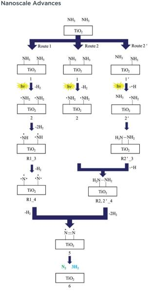
Fig. 4 The suggested reaction mechanism for decomposition of NH<sub>3</sub> to N2 and H2 over TiO2 photocatalysts. Reprinted from ref. 39, Copyright 2017, with permission from Elsevier.
