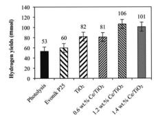
Fig. 5 Hydrogen yields over each investigated photocatalyst and in the case of photolysis after 10 h irradiation. Conditions: 10 h of irradiation, 8 W Hg lamp (254 nm), 100 mL of NH<sub>4</sub>OH, 0.1 g of the photocatalyst. Reprinted from ref. 40. Copyright 2015, with permission from Flsevier
