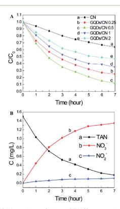
Fig. 10 (A) Effects of the  $g-C_3N_4$  and GQDs/CN composite dosage on the photocatalytic treatment of TAN solution. (B) Concentration changes of TAN,  $NO_2^-$  and  $NO_3^-$ . Reproduced from ref. 49 with permission from the Royal Society of Chemistry.
