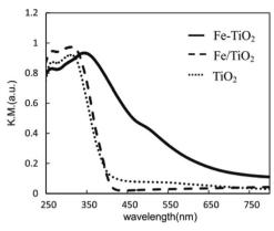
Fig. 6 UV-vis-DR spectra of Fe-TiO $_2$ , Fe/TiO $_2$  and TiO $_2$  photocatalysts. Reprinted from ref. 41. Copyright 2015, with permission from Elsevier.
