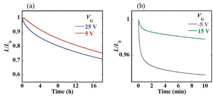
Fig. 5 (a) The operational lifetime of the red QD-HLET tested at different  $V_{GS}$  and a constant current density of 71 mA cm<sup>-2</sup>. (b) The luminance as a function of time for the red QD-HLET with a loop test between -5 V and 15 V of  $V_{GS}$  at a constant current density of 71 mA cm<sup>-2</sup>.
