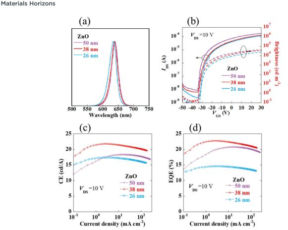
Fig. 6 (a) The EL spectra, (b) electronic and optical transfer characteristic curves, (c) CE versus current density curves, and (d) EQE versus current density curves of red-QD-HLETs with a ZnO-nanoparticle thickness of 50 nm, 38 nm and 26 nm, respectively, measured at  $V_{DS} = 10 \text{ V}$ .
