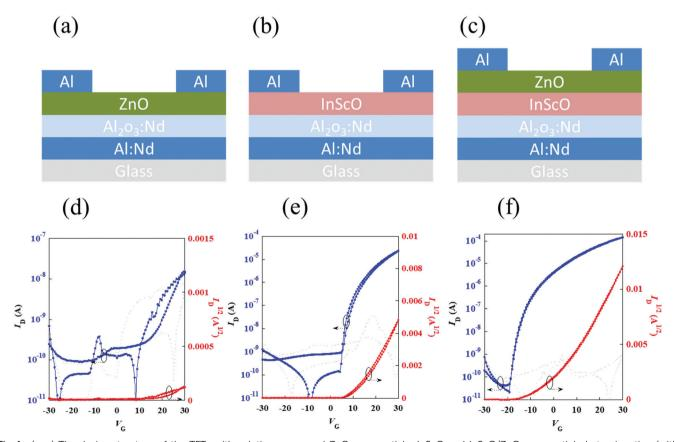
Fig. 1 (a-c) The device structure of the TFTs with solution-processed ZnO-nanoparticle, InScO and InScO/ZnO-nanoparticle heterojunction (with optimized thicknesses of 3.4 nm/50 nm) channels by spin-coating, respectively. (d-f) The transfer characteristics of TFTs with different channels measured at  $V_{\rm DS}$  = 30 V and  $V_{\rm GS}$  = -30 to 30 V.
