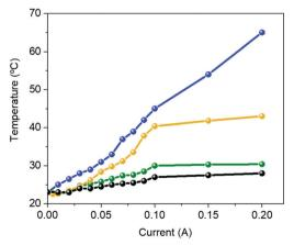
Fig. 4 Changes in the temperature vs. applied current for a commercial 450 nm LED (black) and Bio-HLEDs with FP-polymer (blue), FP-SF (orange), and SF (green) bio-phosphors.
