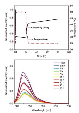
Fig. 6 Thermal stability of FP-SF bio-phosphors at a constant temperature (50 °C) for 24 h and after cooling, monitoring the emission intensity (top), and emission band shape (bottom) upon excitation with a blue LED (450 nm) for 5 s every 10 min
