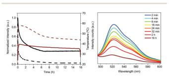
Fig. 5 Typical performance of 'on-chip' Bio-HLEDs operating at highapplied currents of 200 mA. Left: Overall emission intensity decay (black) along with the temperature changes (red) over time for Bio-HLEDs with FP-SF (solid line) and FP-polymer (dashed line). Right: Electroluminescence spectra of Bio-HLEDs with FP-SF phosphors over time.
