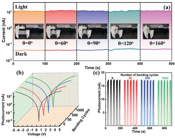
Fig. 4 (a) Output currents of the device with different bending angles under dark and light illumination with a light intensity of 0.2 mW cm<sup>-2</sup> at a bias voltage of 5 V. The insets are the corresponding optical images of the device under five bending states.  $\theta$  is the bending angle. (b) I-V and (c) I-V the device under different bending cycles.
