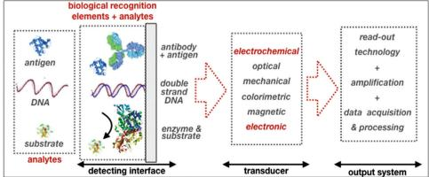
Fig. 1 A schematic of the elements and the single components that are comprised in a typical biosensor
