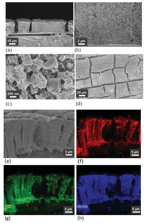
Fig. 4 (a-c) SEM cross-section views at different magnifications of AI/VACNT/ZnO/perovskites and (d) top view of the deposit. (e) SEM cross-section of Al/VACNTs/ZnO/perovskite and associated EDX analysis. (f) Carbon repartition, (g) Zn repartition and (h) Pb repartition. These pictures show the efficient colocalization of CNTs, ZnO and perovskite.
