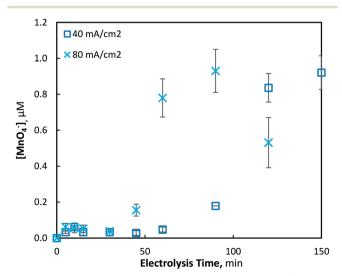
Fig. 8 Production of permanganate at 40 and 80 mA cm<sup>-2</sup> over 120 min of electrolysis (pH = 7,  $[Mn^{2+}]_0$  = 175  $\mu$ M, T = 21.0  $\pm$  0.8 °C).
