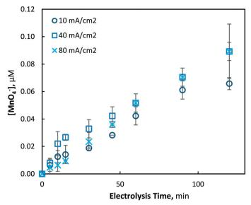
Fig. 9 Permanganate production under 10, 40 and 80 mA cm<sup>-2</sup> electrolysis conditions over 120 min (pH = 7, [Mn<sup>2+</sup>]<sub>0</sub> = 39  $\mu$ M,  $T = 21.0 \pm 0.8$  °C).
