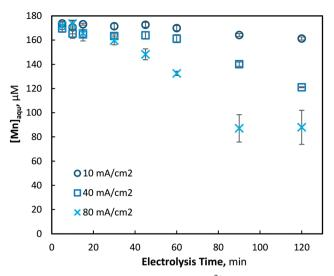
Fig. 2 Removal of aqueous manganese (Mn<sup>2+</sup>) with electrolysis time and current densities of 10, 40 and 80 mA cm<sup>-2</sup> (pH = 7,  $[Mn^{2+}]_0$  = 175  $\mu$ M,  $T = 21.0 \pm 0.8 \circ$ C).
