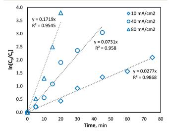
Fig. 4 Indirect quantification of hydroxyl radical formation (methanol degradation) with current densities of 10, 40 and 80 mA cm<sup>-2</sup> (pH = 7,  $T = 21.0 \pm 0.8 \, ^{\circ}\text{C}$ ).
