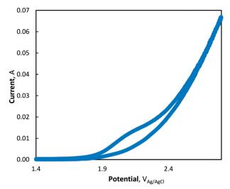
Fig. 3 Cyclic voltammogram of MnCl<sub>2</sub> at pH = 7 (phosphate buffer) and 10 mV s<sup>-1</sup> scan rate.
