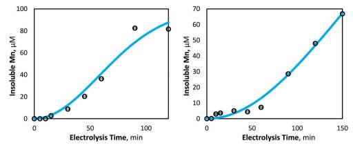
Fig. 7 Model and experimentally yielded results of insoluble manganese (Mn<sup>3+,4+</sup>) generation at 80 mA cm<sup>-2</sup> (left) and 40 mA cm<sup>-2</sup> (right) (pH = 7,  $[Mn^{2+}]_0 = 175 \mu M, T = 21.0 \pm 0.8 \circ C).$
