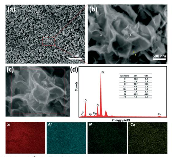
Fig. 3 (a) and (b) SEM images of Cu<sup>2+</sup>@POSS\_SWy-2. (c) SEM image with the area selected for energy dispersive X-ray spectroscopy (EDS) spectra and EDS elemental mapping measurement marked in red. (d) SEM-EDS spectra of  $Cu^{2+}$ @POSS\_SWy-2. Inset: The elemental composition results. The bottom panels show the EDS elemental mapping results for Si, Al, N and Cu in  $Cu^{2+}$ @POSS\_SWy-2 based on the red square area in (c).
