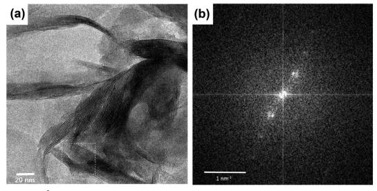
Fig. 2 (a) TEM image of Cu<sup>2+</sup>@POSS\_SWy-2. (b) Fast Fourier transform (FFT) of the square marked in white. An interlayer distance of 17.9 Å is deduced from this graph.
