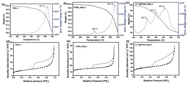
Fig. 4 Thermogravimetric analysis (TGA) and differential thermal analysis (DTA) data for (a) SWy-2, (b) POSS\_SWy-2 and (c) Cu<sup>2+</sup>@POSS\_SWy-2. N<sub>2</sub> adsorption-desorption isotherms of SWy-2 (d), POSS\_SWy-2 (e) and Cu<sup>2+</sup>@POSS\_SWy-2 (f).
