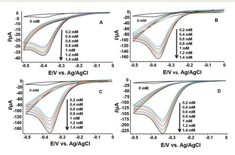
Fig. 5 Electrochemical reduction of H<sub>2</sub>O<sub>2</sub> (various concentrations) on (A) bare GC electrode, (B) GC electrode modified with H<sub>2</sub>L, (C) GC electrode modified with compound 1, and (D) GC electrode modified with compound 2.
