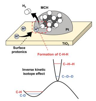
Fig. 16 Schematic image of MCH dehydrogenation facilitated by surface protonics, and inverse kinetic isotope effect.
