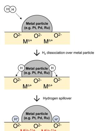
Fig. 1 Schematic images of spillover of H atoms from metal particles to reducible metal oxides.
