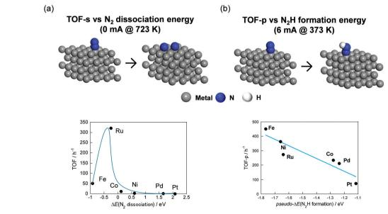
Fig. 15 Illustration of DFT calculation models and relation between TOF-s without the electric field and  $N_2$  dissociation energy (a), TOF-p with the electric field, and  $N_2$ H formation energy (b).
