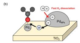
Fig. 2 Schematic image of the ketone/aldehydes hydrogenation over Pd $_1/\text{TiO}_2$  (a) and Pd $_{1+\text{NPs}}/\text{TiO}_2$  (b).
