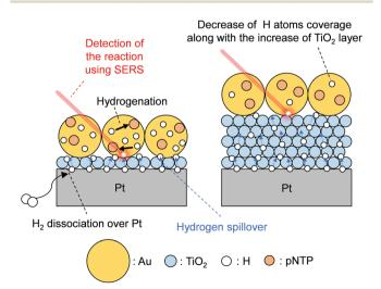
Fig. 9 Schematic image of hydrogen spillover on a Au/TiO $_2$ /Pt sandwich sample.
