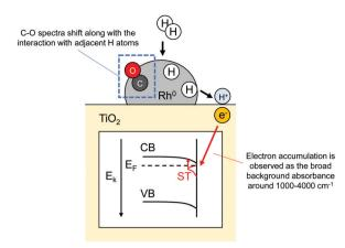
Fig. 7 Illustration of FT-IR measurement for detecting H atoms adsorption over Rh<sup>0</sup> and n-doping into TiO<sub>2</sub>.
