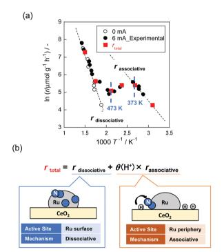
Fig. 13 Temperature dependence of  $NH_3$  synthesis rate (r) without the electric field ((a), open plot), in the electric field ((a), black closed plot) and overall reaction rate ((a), red closed plot), calculated based on the concept shown in (b).
