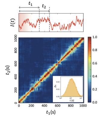
Fig. 4 Two-time correlation function  $c_2(Q,t_1,t_2)$  of deeply supercooled water originating from high density amorphous (HDA) ice at T = 120 K, which is near the glass transition temperature of HDA. One can see that the dynamics are highly heterogeneous from the fluctuations along the diagonal. The corresponding dynamic susceptibility determined by  $c_2$ shown in the inset, which is a quantitative measure of dynamical heterogeneity (adapted with permission from ref. 53).
