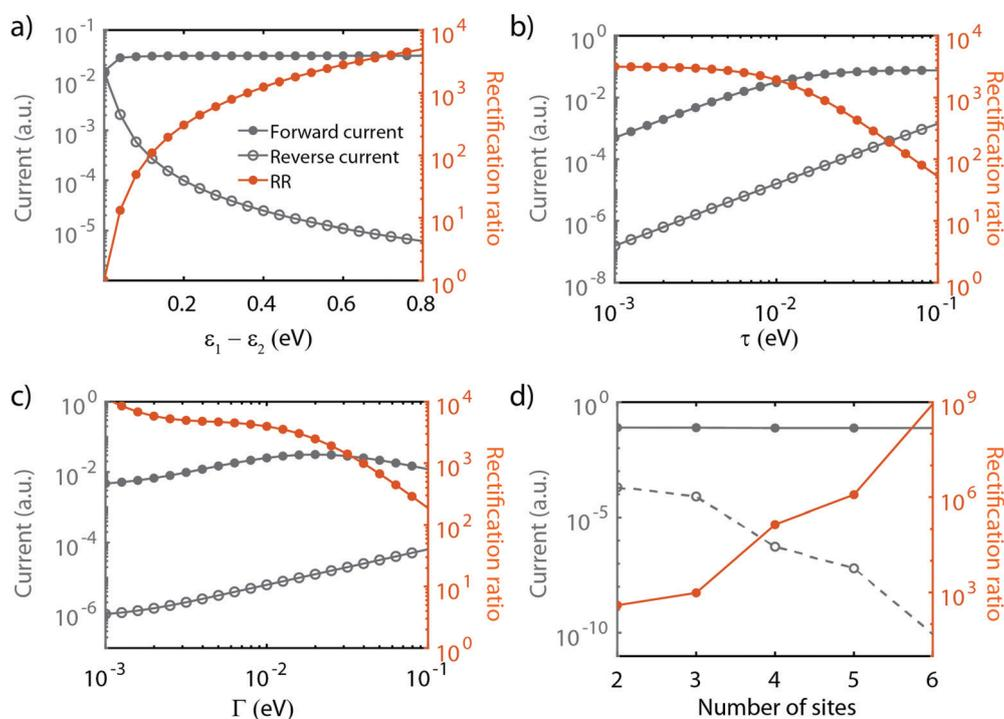
Fig. 4 Influence of the model parameters on the current and rectification ratio. Influence of (a) on-site energies, (b) inter-site coupling  $\tau$ , (c) electronic coupling  $\Gamma$  on the two-site model and (d) the effect of increasing the number of sites. Fixed parameters (when not varied):  $\varepsilon_1 = 0.25$  eV,  $\varepsilon_2 = -0.25$  eV,  $\alpha_{1,2} = 0.25$ ,  $\tau = 10$  meV and  $\Gamma_{L,R} = 25$  meV.
