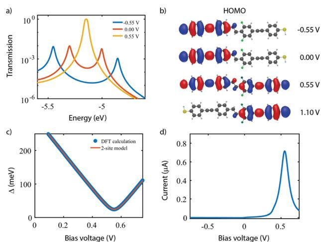
**Fig. 9** DFT + NEGF calculations on the asymmetric DPE molecule. (a) Electron transmission as a function of electron energy for different bias voltages. (b) Energy splitting  $\Delta$  as a function of bias voltage. (c) Isosurface of the HOMO for different bias voltages. (d) Current-voltage characteristic calculated for the HOMO being aligned with the Fermi energy.
