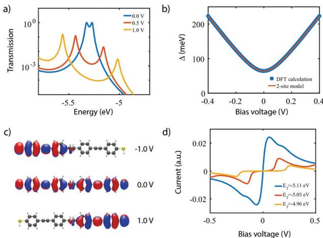
Fig. 6 DFT + NEGF calculations on the symmetric DPE molecule (2). (a) Electron transmission for different bias voltages. (b) Energy splitting  $\Delta$  as a function of bias voltage. The solid orange line is a fit to the two-site model, yielding  $\alpha = 0.53$ ,  $\tau = 32$  meV and  $\epsilon_1 - \epsilon_2 = 0$  eV. (c) Isosurface of the HOMO for different bias voltages. (d) Current–voltage characteristic for different positions of the Fermi energy.
