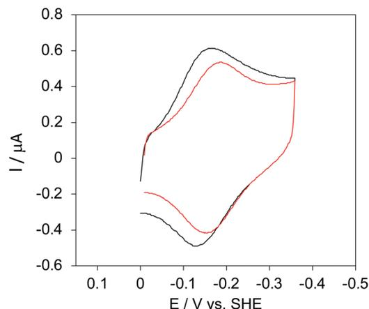
Fig. 6 Cyclic voltammograms for the M80A variant of yeast iso-1-cytochrome c in the presence of varying urea concentrations at pH 7.2 under diffusive conditions. 0 M urea (red) and 6 M urea (black). Working electrode: polycrystalline gold wire functionalized with 4-mercaptopyridine. Working solution: 10 mM phosphate buffer plus 100 mM sodium perchlorate, pH 7.2.  $T = 293$  K. Sweep rate:  $0.5 \text{ V s}^{-1}$ . Similar CVs were obtained for the M80A/Y67A variant.
