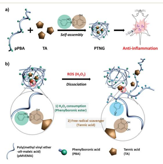
Scheme 1 (a) Preparation and administration of self-assembled PTNG and (b) illustration of combinatorial ROS-scavenging effects of PTNG; the phenylboronic ester bond consumes  $H_2O_2$ , and TA scavenges the free radical, respectively.
