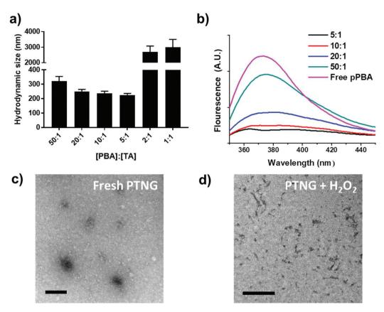
Fig. 1 Characterization of PTNG. (a) Hydrodynamic size of PTNG and (b) intrinsic fluorescence of PBA varying with the ratio of PBA and TA. TEM image of PTNG (c) without  $H_2O_2$  and (d) after treating with  $H_2O_2$  (scale bars = 200 nm and 100 nm, respectively).
