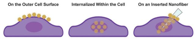
Scheme 2 Three approaches for performing SERS experiments with cells, where the plasmonic nanoparticles can be located at the surface of the cell, internalized within the cell, or on a nanofiber that is then inserted into the cell.
