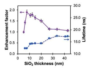
Fig. 7 Fluorescence enhancement factor of silanized methoxyquinolinium (MQ,  $\lambda_{\rm ex}$  = 340 nm,  $\lambda_{\rm em}$  = 440 nm) and related lifetime ( $\lambda_{\rm ex}$  = 308 nm) in In@(RB)@SiO2@MQ architectures as a function of spacer thickness. Reproduced from ref. 103 with permission from the Royal Society of Chemistry, Copyright 2017.
