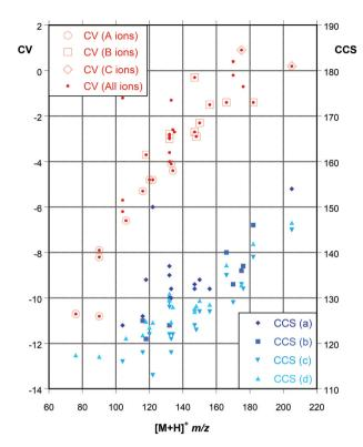
Fig. 2 CV and CCS as a function of m/z for a selected set of AAs and related species (see list in Table S4†). CV values (in V), 1 V corresponding to an electric field of 1.43 kV m<sup>-1</sup> or ~0.07 Td. CCS (in Ų) are taken from (a) ref. 38, (b) ref. 33, (c) ref. 17, and (d) ref. 51.
