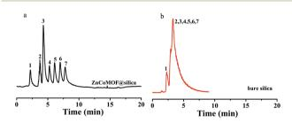
**Fig. 2** Chromatograms for the separation of seven carbohydrates on ZnCoMOF@silica (a) and bare silica (b): L-rhamnose monohydrate (1), D-ribose (2), D-fructose (3), sucrose (4), lactose (5), melezitose (6) and raffinose (7) mobile phase: 90% acetonitrile, 10% water; flow rate = 0.8 mL min $^{-1}$ , T = 25 °C. ELS detector: gas flow: 4 L min $^{-1}$ , tube temperature 115 °C.
