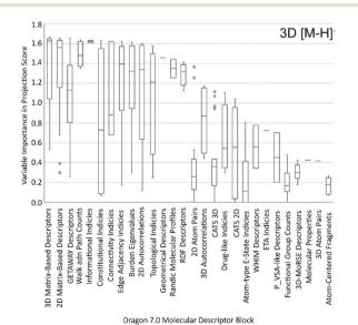
Fig. 2 Each molecular descriptor used in the 3D [M - H] model belongs to a block as defined by the Dragon 7.0 software. The box and whisker plot show the range of Variable Importance in Projection (VIP) scores given for each block. The higher the VIP score the more important the variable is to the multivariate model.
