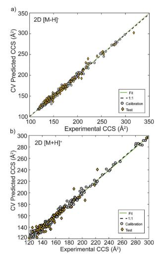
Fig. 1 Measured vs. cross-validation (CV)-predicted CCS for metabolites developed using (a) 2D structural files to calculate molecular descriptors for  $[M - H]^-$  adducts, and (b) 2D structural files to calculate molecular descriptors for [M + H]+ adducts. Optimal molecular descriptors were selected by a genetic algorithm.
