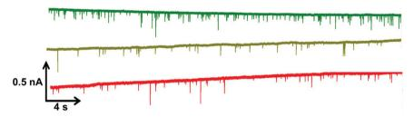
Fig. 2 Example data sets for DNA blank S-beads (green), S-beads incubated with 50 nM PrP<sup>C</sup> (olive) and 100 nM PrP<sup>C</sup> (red). Magnified section of this are also shown in Fig. s1.† N.B. the blank beads have been run prior to dilution.
