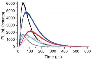
Fig. 5 Time-resolved PL intensities ( $\lambda_{em}=542\pm10$  nm) of UCNP-DNA nanohybrids without (no FRET) and with (FRET) 3.54 nmol mg $^{-1}$  Cy3.5-ssDNA. Black/gray: c-UCNP-DNA without/with Cy3.5-ssDNA ( $\lambda_{ex}=980$  nm); blue/cyan: css-UCNP-DNA without/with Cy3.5-ssDNA ( $\lambda_{ex}=980$  nm); red/rose: css-UCNP-DNA without/with Cy3.5-ssDNA ( $\lambda_{ex}=980$  nm);
