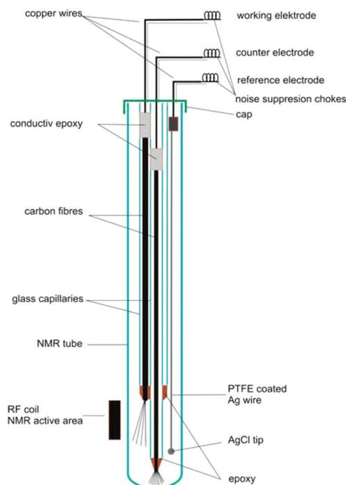
**Fig. 14** Schematic of a three-electrode NMR-SEC cell with carbon fibre WE and CE, partially placed in the NMR detection area. Reprinted with permission from Klod *et al.*<sup>253</sup> Copyright 2009 American Chemical Society.
