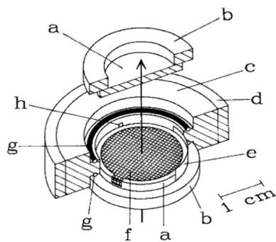
**Fig. 2** Schematic representation of the IR-SEC cell. The arrow represents the propagation of the IR-light beam (a) IR-transparent  $\text{CaF}_2$  window mounted onto a (b) Plexiglas ring, (c) Teflon body, (d) steel surround, (e) Pt counter electrode, (f) the mesh working electrode, (g) O-ring, (h) capillary connection to the reference electrode. Reprinted from the original work by Moss *et al.*,<sup>11</sup> Copyright 1990, with permission from John Wiley and Sons.
