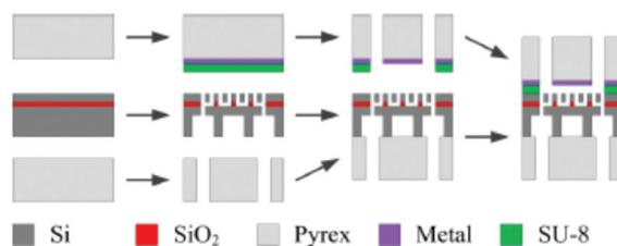
Fig. 25 Membrane fabrication scheme. Reprinted from the original work by Trimarco *et al.*,<sup>308</sup> Copyright 2015, with the permission of AIP Publishing.
