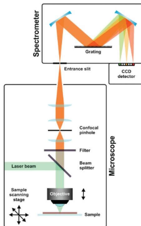
Fig. 9 Schematic representation of a Raman setup. Reprinted from the original work by Schmid and Dariz,<sup>119</sup> Copyright 2019, with permission from Creative Commons. Licensed under CC BY 4.0.
