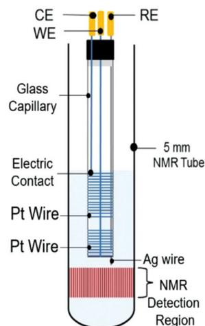
**Fig. 18** Schematic of a coil-based three-electrode NMR-SEC cell. Reprinted from the original work by da Silva *et al.*,<sup>275</sup> Copyright 2019, with permission from Elsevier.
