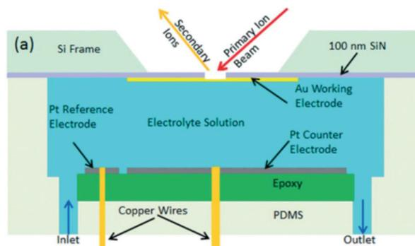
Fig. 26 Schematic of an EC-SIMS cell. Reprinted from the original work by Liu *et al.*,<sup>311</sup> Copyright 2014 – Published by The Royal Society of Chemistry.
