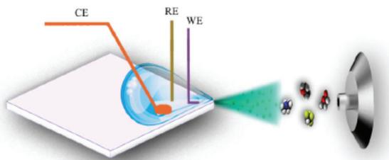
Fig. 21 D Schematic of the droplet-based EC-MS approach. Reprinted with permission from Yu *et al.*<sup>292</sup> Copyright 2018 American Chemical Society.
