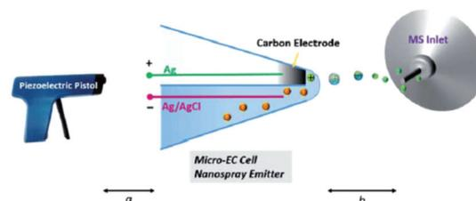
Fig. 22 Schematic of the thin-layer double-barrel capillary setup. Reprinted from the original work by Qiu *et al.*,<sup>294</sup> Copyright 2016, with permission from Creative Commons. Licensed under CC BY 3.0.
