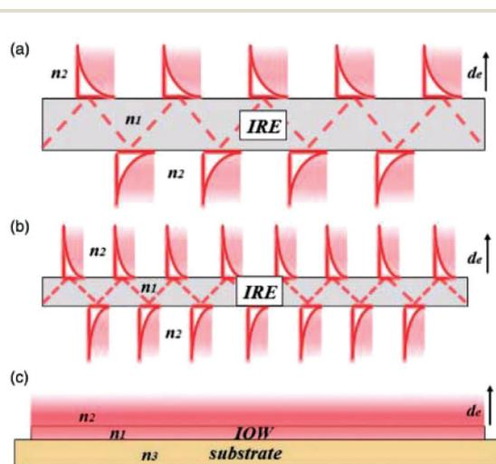
**Fig. 8** Schematic representation of the evanescent wave/field with an ever decreasing IRE thickness. As one can see in (a) and (b), the smaller IRE has more reflections than the bigger IRE. When the size is small enough, as one can see in (c), a waveguide is created with a continuous evanescent field. Reprinted from the original work by Schadle and Mizaikoff,<sup>68</sup> Copyright 2016, with permission from SAGE Publications.
