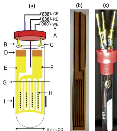
**Fig. 16** Schematic and photograph of an NMR-SEC cell with interdigitated WE and CE placed in the NMR detection area. Reprinted from the original work by Sorte *et al.*,<sup>269</sup> Copyright 2016, with permission from Elsevier.
