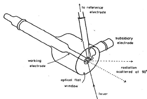
**Fig. 10** Example of a stationary electrochemical cell used for Raman experiments. Reprinted from the original work by Fleischmann *et al.*,<sup>120</sup> Copyright 1974, with permission from Elsevier.
