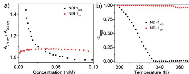
Fig. 3 Comparison of the (a) CAC and (b) thermal stability of NDI-1<sub>agg</sub> (aggregated spontaneously) and NDI-1<sub>sp</sub> (prepared by CSP of NDI-1<sub>mono</sub> using 10% DBU).  $A_{375}$  and  $A_{356}$  indicate absorption at 375 and 356 nm, respectively, in the UV/Vis spectra in decane [ $l = 1$  cm;  $C = 1 \times 10^{-4}$  M];  $\alpha_{agg}$  at each temperature was calculated from the variable temperature UV/Vis spectra (Fig. S5†).
