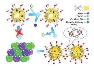
Scheme 2 The detailed assembly process of nanocage architecture 2 from discrete nanocage 1 and the nanocage dimer.
