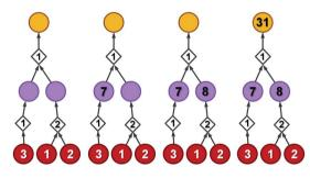
Fig. 4 A simple example illustrating bottom-up propagation of costs. All reactions have the same yield of 50%. Costs of starting materials (per mmol) are given by the numbers in the red nodes. Fixed costs of synthetic operations are indicated inside the diamond-shaped reaction nodes. For details of the calculations, see the main text.
