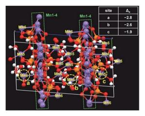
Fig. 4 The unit cell of the MnPi used to calculate the preference of the oxidation of different Mn sites. The three Mn sites that can be most easily oxidized are marked with the yellow circles. The corresponding charge differences of these Mn sites after the removal of one electron are listed in the table.
