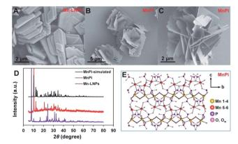
Fig. 2 The SEM images of the as-prepared Mn-LNPs (A) and MnPi (B and C). (D) XRD patterns of the as-prepared Mn-LNPs and MnPi, and simulated XRD patterns of MnPi from crystal structure data. (E) The crystal structure of MnPi with six different Mn sites, including Mn(1–4) layers and out-of-plane Mn(5,6) centres.
