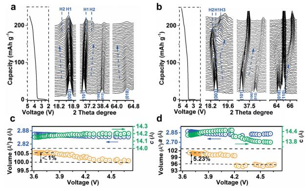
Fig. 4 Structural evolution of LiNi<sub>0.9</sub>Co<sub>0.07</sub>Mg<sub>0.03</sub>O<sub>2</sub> (a and c) and NCM811 (b and d). (a and b) In situ XRD patterns at selected  $2\theta$  regions and the corresponding galvanostatic curves on first charging. (c and d) The variation of lattice parameters and cell volumes as a function of voltage.
