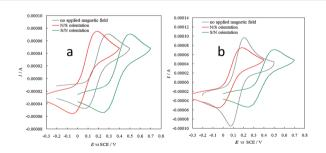
Fig. 7 CV patterns for the achiral  $Fe(CN)_6^{3-}|Fe(CN)_6^{4-}|$  redox couple, recorded at 0.05 V s<sup>-1</sup> in aqueous solution on ITO electrodes (a) or SWCN SPEs (b) modified by a thin layer of (*P*)-enantiopure oligo-7-TH thin film, as such and under application of an external magnet with N/S or S/N orientation (red or green lines respectively).
