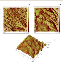
Fig. 8 Tapping Mode AFM images (a)  $10 \times 10~\mu\text{m}^2$ , (b) and (c)  $4 \times 4~\mu\text{m}^2$  of BT<sub>2</sub>T<sub>4</sub> oligomers electrochemically deposited onto uflat-ITO electrode by 2 voltammetric cycles at  $0.2~\text{V s}^{-1}$  from a DCM solution of 1.7 mM racemic monomer BT<sub>2</sub>T<sub>4</sub>.
