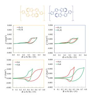
Fig. 9 Enantioselection performance of enantiopure (S)-BT<sub>2</sub>T<sub>4</sub> (yellow) and (R)-BT<sub>2</sub>T<sub>4</sub> (blue) films towards chiral electroactive ferrocenyl probes, named (S)-Fc and (R)-Fc, in DCM (top) and ACN (bottom) as solvents.
