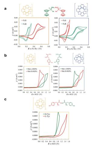
Fig. 6 Enantioselection performance of enantiopure (P)-7-TH (yellow box) and (M)-7-TH (blue box) electrode surfaces towards chiral electroactive (a) ferrocenyl probes, named (S)-Fc and (R)-Fc, (b) methyl L-and D-DOPA and (C) L- and D-tyrosine. CVs were recorded at 0.05 V s<sup>-1</sup> potential scan rate.
