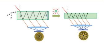
Fig. 5 Proposed schematic illustration of using  $Zn(CH_3COO)_2 \cdot 2H_2O$  crystals as a sensing medium in a Fabry–Perot interferometer pressure sensor by taking advantage of its large NAC.
