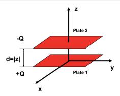
Fig. 1 Schematic view of a parallel-plate nanocapacitor consisting of two identical plates, 1 and 2 placed face-to-face a distance, d=|z| apart. The two plates of the nanocapacitor are assumed to be identical squares with length, L. The plates contain, respectively, a total charge of  $\pm Q$  which is considered uniformly spread over the surface area resulting in a uniform surface charge density,  $\pm Q/L^2$ .
