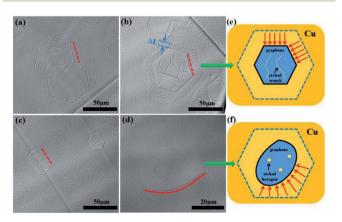
Fig. 3 Optical microscopy images of graphene domains after etching at 1000 °C for (a and b) 10 and (c) 15 min. The gas flow rate of etching was 2:50 (20 sccm  $\rm H_2$  and 500 sccm Ar). (d) Optical microscopy image of GED at 1050 °C. (e and f) Schematics of different etching results between GECRP and GED.
