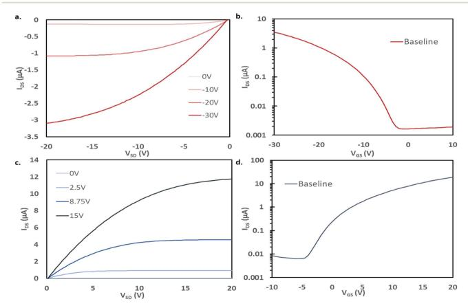
Fig. 2 Output and transfer curves for baseline BGBC OTFTs tested at 25 °C. (a) Output curve and (b) transfer curve ( $V_{DS}=-20$  V) for CuPc devices. (c) Output curve and (d) transfer curve ( $V_{DS}=20$  V) for  $F_{16}$ -CuPc devices.
