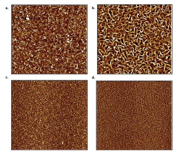
Fig. 5 AFM images of CuPc (a and c) and  $F_{16}$ -CuPc (b and d) thin films deposited on  $SiO_2$  substrates at 140 °C (a and b) and 20 °C (c and d). Images (a and b) are 5  $\mu$ m  $\times$  5  $\mu$ m while (c and d) are 2.5  $\mu$ m.
