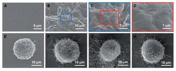
Fig. 2 (A and E) ESEM images of the flat films with surfaces which do not have a microstructure and the PC3 cell, which displayed a spherical shape and does not have enough filopodia. (B–D) ESEM images of the rGO film surface which clearly show the existence of a petal-like wrinkled architecture. (F–H) The attachment relationship between a 22Rv1 cell, a PC3 cell and an mCRPC cell and the functional surface with the cell shape changed and the appearance of filopodia.
