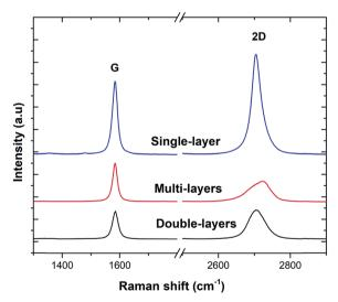
Raman spectra of 3D-GF obtained at different positions.
