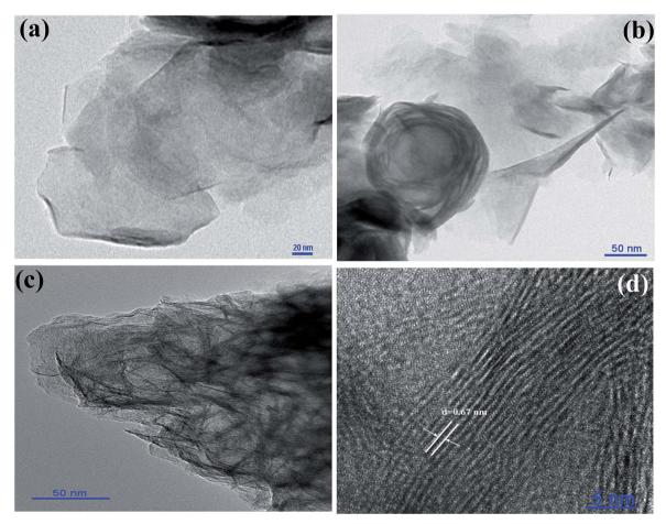
Fig. 2 (a)-(d) show the TEM images of MoS<sub>2</sub>. d-Spacing between the MoS<sub>2</sub> layers shown in figure (d) is 0.67 nm.
