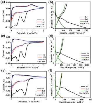
Fig. 5 CV curves of N/S-HCNFs (a), N-HCNFs (b) and N-n-HCNFs (c) at a scan rate of 0.1 mV s<sup>-1</sup>; the first three GCD profiles of N/S-HCNFs (d), N-HCNFs (e), and N-n-HCNFs (f) at  $0.05 \text{ A g}^{-1}$ .
