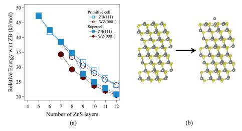
Fig. 3 (a) Relative energies for ZnS WZ(0001) and ZB(111) films, based on calculations using both a primitive cell and a surface  $2 \times 2$  supercell. (b) Schematic representation of the initial and the optimised ZnS ZB(111) film showing the surface reconstruction by expulsion of a Zn atom. Zn atoms are grey and S atoms are yellow.
