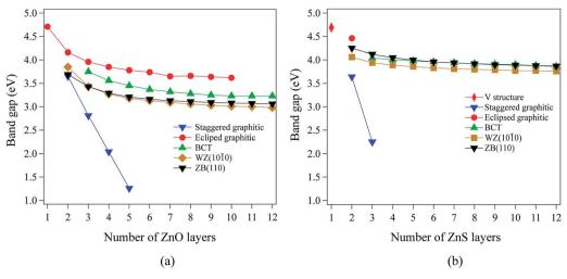
Fig. 4 Band gaps as a function of film thickness for non-polar (a) ZnO and (b) ZnS films.
