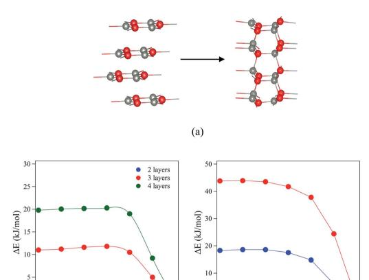
Fig. 9 (a) Staggered graphitic and WZ(1010) structures. (b and c) Energy profiles of the structural transitions for (b) ZnO and (c) ZnS (staggered graphitic → WZ(1010)). All energies are relative to the final state. Zinc atoms are grey, oxygens red, and sulphurs yellow.
