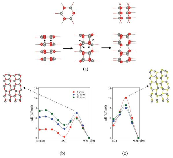
Fig. 8 (a) Structures and indications of atomic movements required for transitions from eclipsed graphitic to WZ(1010) via a BCT structure. (b and c) Energy profiles of the structural transitions for (b) ZnO (eclipsed graphite  $\rightarrow$  BCT  $\rightarrow$  WZ(1010)) and (c) ZnS (BCT  $\rightarrow$  WZ(1010)). All energies are relative to the final state. Zincs are grey, oxygens red, and sulfurs yellow.
