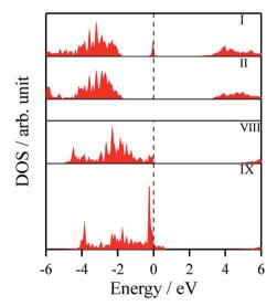
Fig. 7 Partial density of states (PDOS) per layer for polar ZB(111) for ZnS with 9 layers. A similar figure but expanded with PDOS plots for all the layers are given in the ESI. $\dagger$
