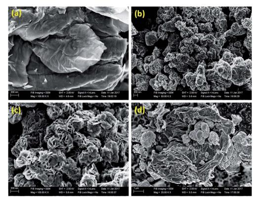
Fig. 3 FESEM images of (a) rGO, (b & c) MoS<sub>2</sub> at different magnifications and (d) MoS<sub>2</sub>@rGO composite.
