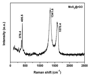
Fig. 2 Raman spectrum of MoS<sub>2</sub>@rGO composite.
