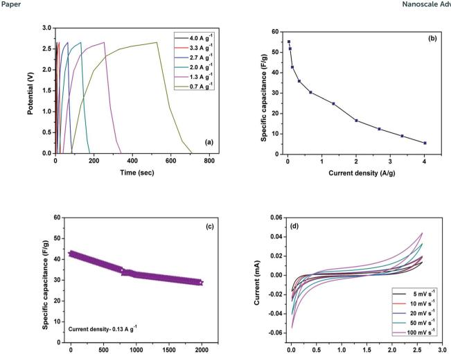
Fig. 6 Electrochemical performance of the symmetric hybrid device (full cell). (a) Galvanostatic charge-discharge curves; (b) specific capacitances at different current densities; (c) cycling performance; (d) cyclic voltammograms at different scan rates.
