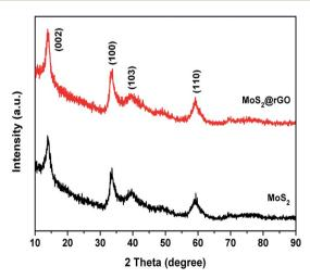
Fig. 1 XRD patterns of MoS<sub>2</sub> and MoS<sub>2</sub>@rGO composite.
