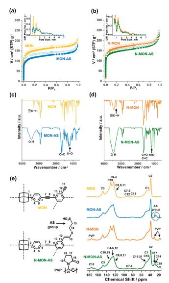
Fig. 3 (a and b) N<sub>2</sub> adsorption-desorption isotherm curves obtained at 77 K and pore size distribution diagrams based on the density functional theory (DFT) method, (c and d) IR absorption, and (e) solid state <sup>13</sup>C NMR spectra of MON, MON-AS, N-MON, and N-MON-AS.
