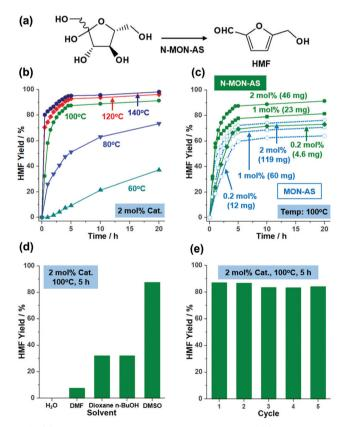
Fig. 4 (a) A scheme of fructose conversion to HMF. (b) Temperaturedependent catalytic performance of N-MON-AS. (c) Comparison of the catalytic performance of MON-AS (0.284 mmol SO<sub>3</sub>H per g) and N-MON-AS (0.731 mmol SO<sub>3</sub>H per g). (d) Solvent-dependent catalytic performance and (e) recyclability of N-MON-AS.
