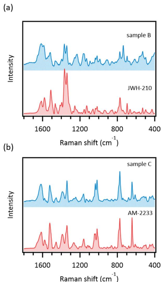
**Fig. 6** Surface-enhanced Raman scattering spectra of methanol extracts of sample B and sample C (in blue). Corresponding spectra of standard solutions are also shown (in red). These spectra were obtained by using a Raman microspectrometer with 1–5 s exposure time.
