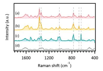
**Fig. 3** Surface-enhanced Raman scattering spectra of a real herbal high. (a) Spectrum obtained from sample A (Table 2), (b) standard spectrum of AM-1220, (c) standard spectrum of AM-2233, and (d) background spectrum. Dashed lines indicate peaks that coincide in the sample and standard spectra. Exposure was 1 s, 100 frames.
