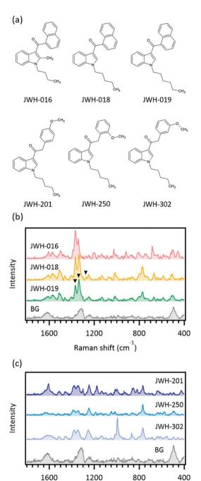
Fig. 2 Measurement of the surface-enhanced Raman scattering spectra of standard solutions. (a) Chemical structures of examined synthetic cannabinoids, (b) spectra of methylene positional isomers, and (c) spectra of methoxy positional isomers. BG indicates the background measurement. Exposure was 1 s, 100 frames. Arrow heads indicate the peaks useful for discrimination.
