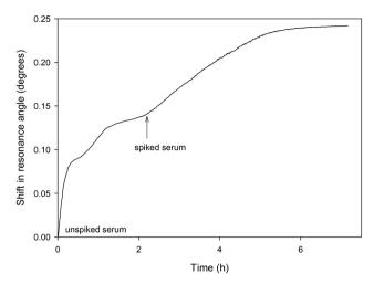
Fig. 6 Shift in resonance angle versus time for a LW sensor functionalised with oligo 2 and reacted with serum diluted to 10% and spiked with 50 nM thrombin
