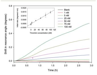
**Fig. 4** Shift in resonance angle *versus* time for different concentrations of thrombin (inset shows the initial rate over the first 5 min *versus* thrombin concentration).
