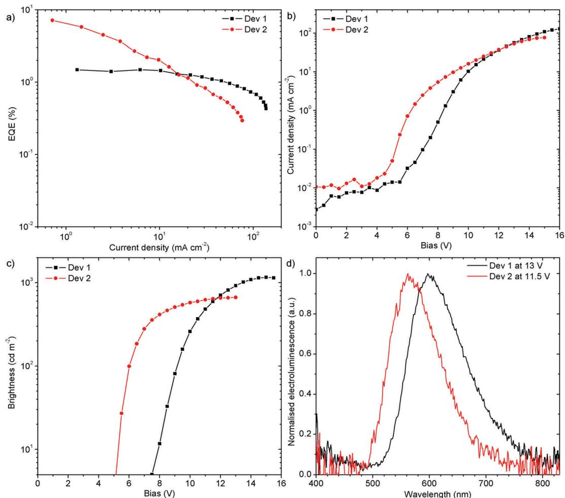
Fig. 11 Electroluminescence characteristics of OLED devices fabricated using **H1-PXZ** and **H2-PXZ** as emitters: (a) EQE vs. current density; (b) current density vs. applied bias; (c) brightness vs. applied bias; (d) electroluminescence spectra. Device structure: ITO | HIL 1.3 N (45 nm) | PVKH (10 nm) | PVK : PBD (60 : 40) co 5% X (32 nm) | TPBi (50 nm) | LiF (0.8 nm) | Al (100 nm). Where X = **H1-PXZ** (Dev 1), X = **H2-PXZ** (Dev 2).
