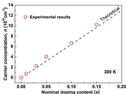
Fig. 2 Carrier concentration as a function of the nominal doping content at room temperature in  $\text{Cu}_3\text{Sb}_{1-x}\text{Sn}_x\text{S}_4$  system. The dashed line is the theoretical model where a full charge transfer is assumed (one hole carrier per dopant).
