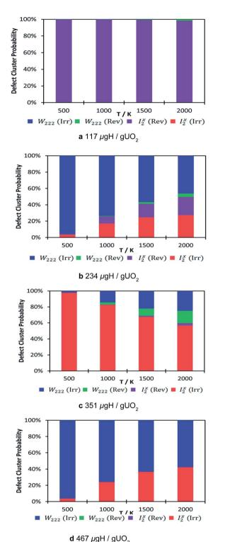
Fig. 5 Defect cluster probability at different local hydrogen concentrations as a function of temperature. The probability has been calculated relative to the most stable cluster for each local hydrogen concentration. Reversible  $W_{222}$  shown in green, irreversible  $W_{222}$  in blue, reversible  $W_{222}$  and irreversible  $W_{222}$  in red.
