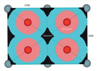
Fig. 2 Representation of hydrogen behavior in UO<sub>2</sub> projected in a [110] direction. Black represents regions where hydride is predicted to be energetically most stable, light blue the H\* radical, pink protonic behavior (i.e. forms a hydroxyl), red the lattice oxygen and blue are the uranium ions. The energies of formation for a hydride or hydroxyl defect by dissolving H<sub>2</sub> gas into UO<sub>2</sub> are shown on the respective regions. Values taken from ref. 35.
