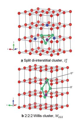
Fig. 1 Structure of oxygen defect clusters in  $UO_2$ . (a) Split di-interstitial  $(l_2^x)$  and (b) 2:2:2 Willis  $(W_{222})$  clusters. Lattice oxygen shown in red.  $U^{4+}/U^{5+}$  are not shown for clarity. Oxygen interstitial  $(O_i'')$  shown in green. Significantly (>10%) displaced lattice oxygen shown in dark blue. Oxygen vacancies  $(V_O'')$  shown in purple. Bonds have been drawn in
