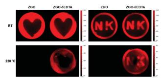
Fig. 7 The information readout by ZGO and ZGO-5EDTA at RT and 220  $^{\circ}\text{C}.$
