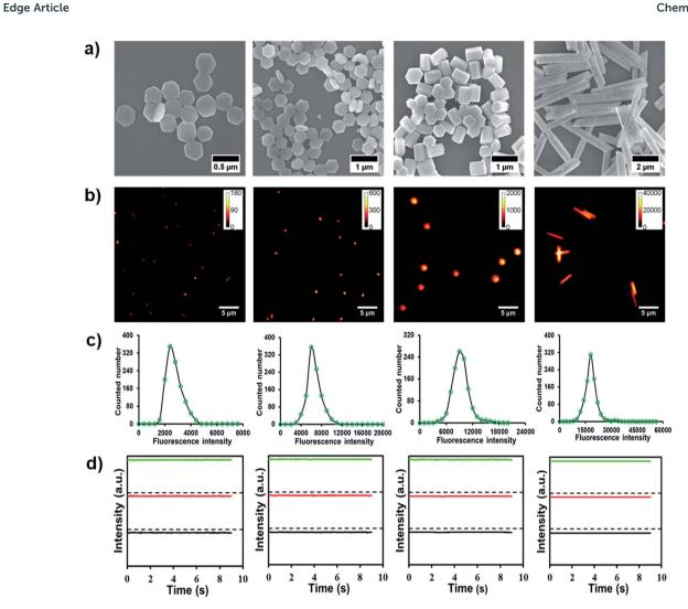
Fig. 1 (a and b) are the SEM and single-particle fluorescence microscopy images of UCNPs-1, -2, -3 and -4. (c) Fluorescence intensity distribution histograms of the corresponding UCNPs. (d) Representative single-particle fluorescence intensity tracks as a function of time in (b).
