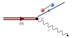
Fig. 11 Diagram representing spontaneous production of correlated exciton–photon pairs from the bare system ground-state  $|0\rangle$ . This process is significant in the ultrastrong coupling regime where lightmatter couplings of the form  $(a_{-\mathbf{k}}^{\dagger}b_{\mathbf{k}}^{\dagger}+\text{h.c.})$  become relevant (see eqn (15))
