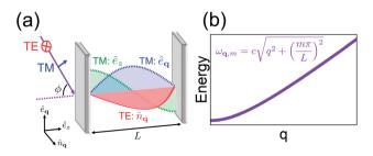
Fig. 1 (a) Representation of microcavity modes excited by radiation (purple) incident at angle  $\phi$ . The electric field polarization of the TE modes (red) lies along  $\hat{n}_{\mathbf{q}}$  while that of TM has  $\hat{\mathbf{e}}_{\mathbf{q}}$  (blue) and  $\hat{\mathbf{e}}_{\mathbf{z}}$  (green, magnitude only) components. (b) Dispersion (energy as a function of mirror-plane wave vector  $\mathbf{q}$ ) of the photonic mode of index m in microcavity with transverse length L.
