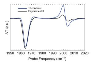
Fig. 9 Experimental and theoretical pump-probe (differential) transmission spectra of strongly coupled W(CO) $_6$  in an optical microcavity. These results correspond to the case where the cavity photon and the molecular vibration (asymmetric C=O stretch) are resonant.
