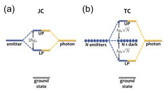
Fig. 2 (a) Jaynes–Cummings (JC) model: emitter and photon strongly couple to form hybridized states termed lower and upper polaritons (LP and UP, respectively) separated in energy by  $2\hbar g_s$ . (b) Tavis–Cummings (TC) model: N emitters interact strongly with a photon to yield polariton (LP, UP) and N-1 dark states. The latter do not couple to light and thus maintain the original emitter energy.
